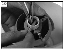
Place ball on downrod. Replace pin removed earlier and pull ball up so that the pin fits in the notches in the ball.
